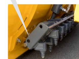
The HK grader is used for the inexpensive, effective maintenance and new construction of water- bound paths, field paths, hiking trails and cycle paths, construction roads or country lanes. It is suitable for spreading and extracting a wide range of bulk materials such as gravel, crushed stone, grand, chippings or sand.
